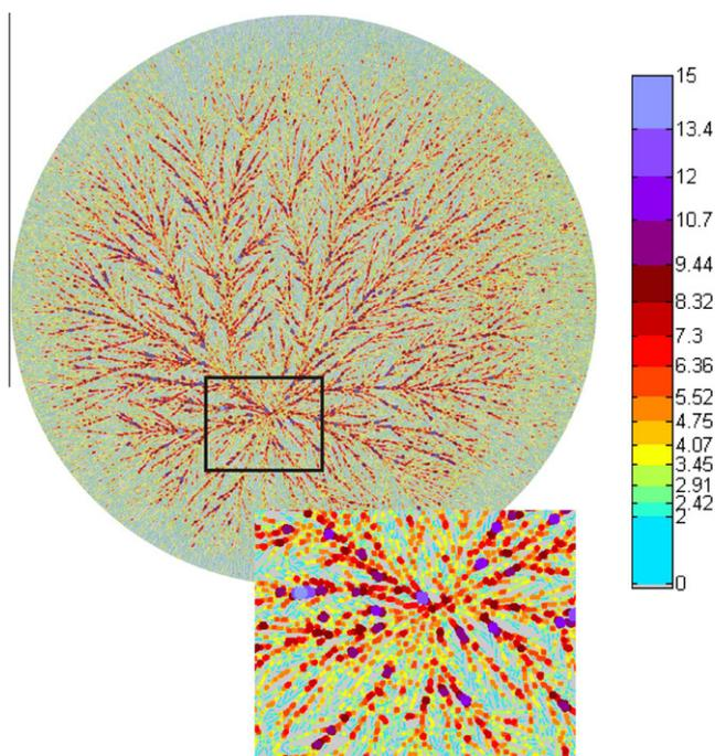
Fig. B.1. Top left: painted droplet representation of the scanned crystallization structure in Fig. A.1, characterized on the basis of the 15 width parameters (top right). Below: enlarged image visualizing the individual painted droplets representing the different width parameters.
